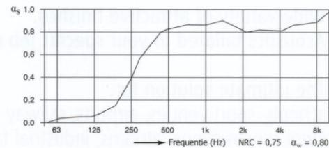
Sound absorption test at the TNO laboratories in The Netherlands. Construction tested directly on hard floor. Thickness of sample 25 mm.
